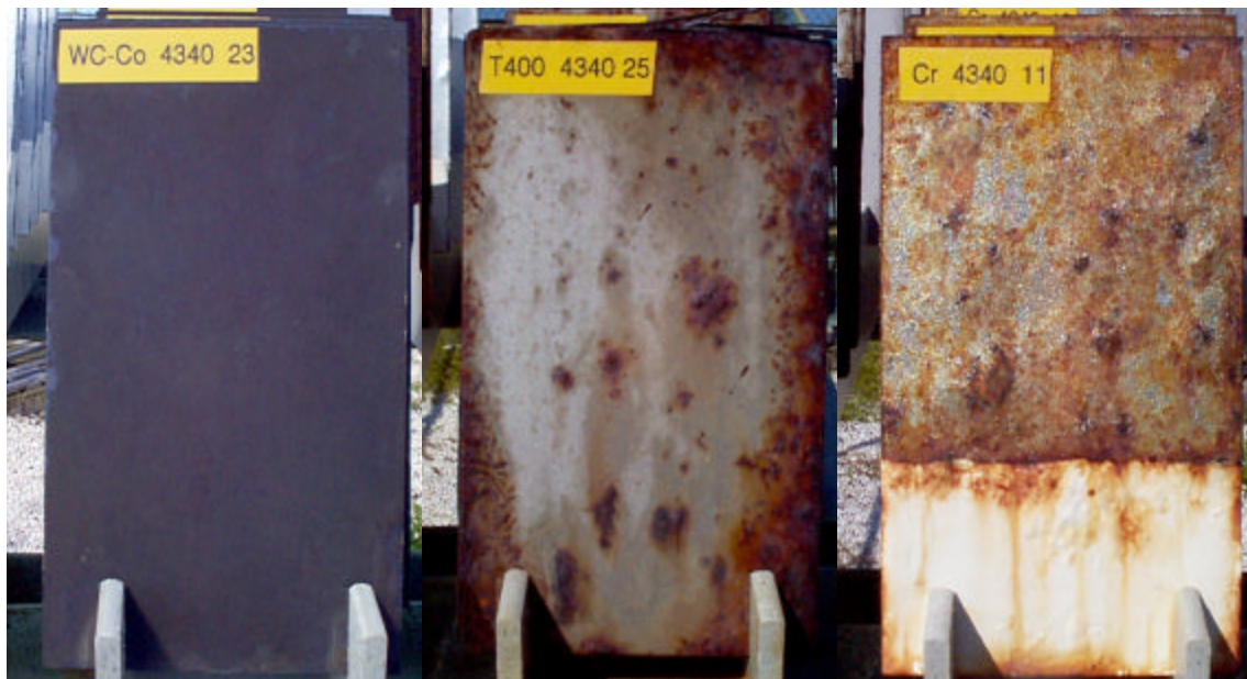
Figure 2. Representative specimens of 4340 steel plates coated with HVOF WC/Co and Tribaloy 400, and hard chrome after 18 months atmospheric exposure plus once weekly spraying with salt water
